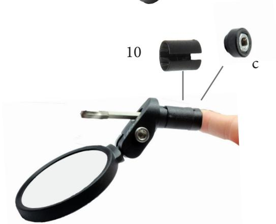
**Step E** - With the expander (10) loose yet secure, insert the bolt end (8,9) into the end of your bike's handlebar. Adjust the angle of the body and mirror to your preferred position and tighten the long screw (6) until the expander(10) has firmly gripped your handlebar. Make sure that the mirror does not obstruct your range of motion and don't forget to wear a helmet!
